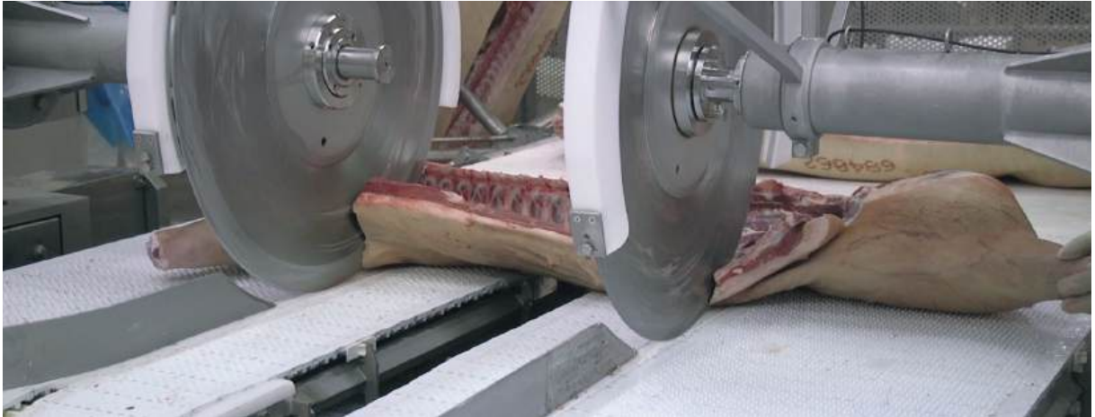
Laserguided primal cutting for pork.
